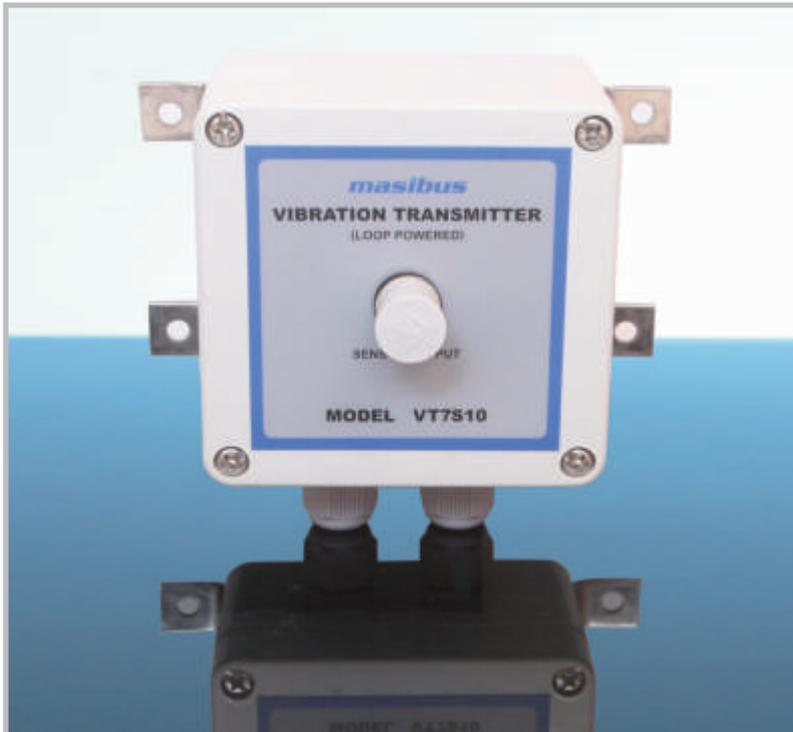
Masibus' Model VT7S10 Vibration Transmitter is an innovative product that excites and reads signal from high temperature accelerometer and transmits overall vibration value with 4-20mA on loop power. It provides output for essential continuous monitoring of critical fan, pump, motor and other industrial machines. It measures the vibration to which it is exposed.
